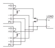
Figure 4-1: N+1 Redundant Operation
