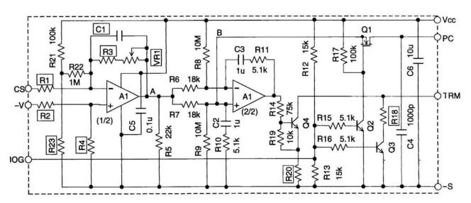
Figure 3-2 Control Circuit fo Parallel Operation
