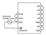
2.5kVAC 1 minute (20mA) (48VDC Input Model: 1.5kVAC)
