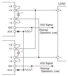
Figure 13-1: Example of IOG Terminal Connection
