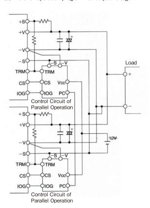
Figure 5-2 Parallel Operation at programmed ouput voltage
