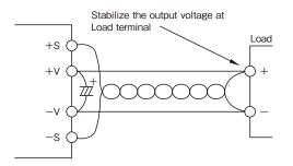
Figure 9-1: Using Remote Sensing
