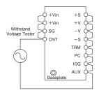
3kVAC for 1 minute (20mA) (24VDC Input model: 2kVAC) Figure21-2: Withstand Voltage Test between Input and output
