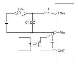
Figure 10-1 Connection of CNT Terminal
