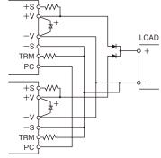
Figure4-2: N+1 Redundant Operation with programmed output voltage
