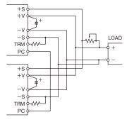
Figure 3-3: Parallel Operation with adjustable voltage
