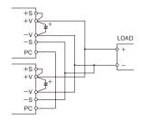
Figure3-1: Parallel Operation
