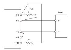
Figure2-2 Example Connection of External Resistance
