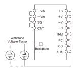
500VDC between output and baseplate for 1 minute Figure21-3: Withstand Voltage Test between output and baseplate
