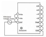
3kVAC 1 minute (20mA) (48VDC Input Model: 1.5kVAC)
