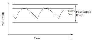
Figure 1-2: Input Ripple Voltage
