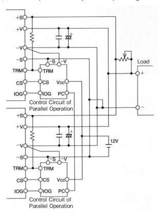
Figure 5-3 Parallel Operation with adjustable output voltage
