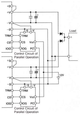
Figure6-1 N+1 Redundant Operation
