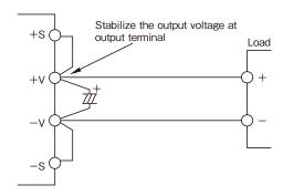
Figure9-2 Remote Sensing Not in Use
