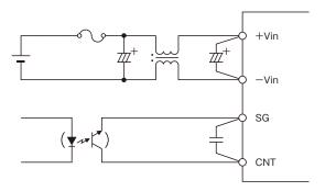
Figure 10-1: Connection of CNT Terminal
