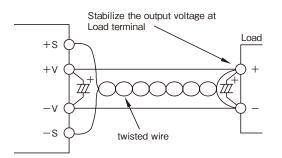
Figure9-1 Remote Sensing at Use
