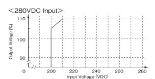
Figure 2-1: Limitation of Input Voltage Range
