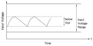
Figure 1-1 Ripple Voltage
