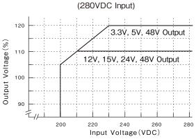
Figure 2-1 Limit of Input Voltage
