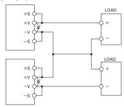
Figure12-2: Series Operation using ± Output
