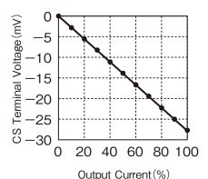
Figure3-3 Characteristics of Output Current vs. CS Terminal Voltage (Example: PH300S48-5)
