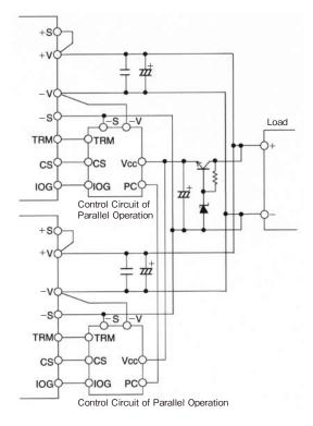
Figure3-5 Example: Vcc is supplied by +V
