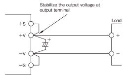
Figure9-2: Without Remote Sensing
