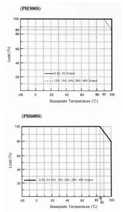
Figure 14-1 Output Derating Curve
