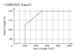
Figure 2-5: Limitation of Input Voltage
