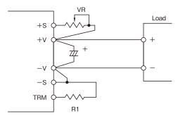
Figure 2-7: Connection Example of External Resistor
