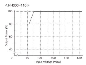
Figure 1-1: PH110 Series Output Derating
