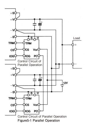
(b) Parallel Operation programmed output voltage
