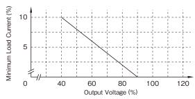
Figure2-6: Minimum Output Current Limit
