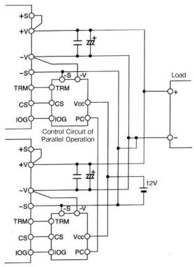
Control Circuit of Parallel Operation
