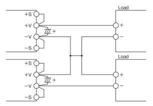
Figure12-2 ±Output Series Operation
