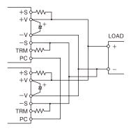
Figure 3-2: Programmed Output Voltage
